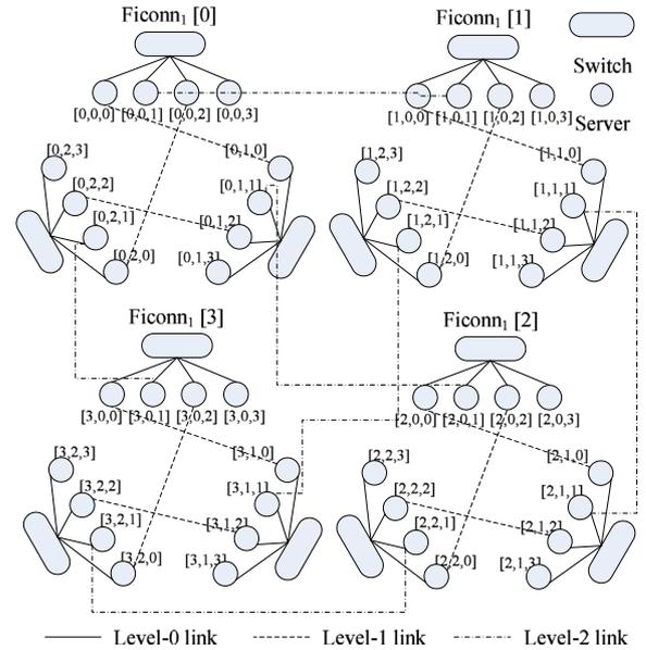
Fig. 24. A FiConn<sub>2</sub> network architecture with  $n = 4$ .
