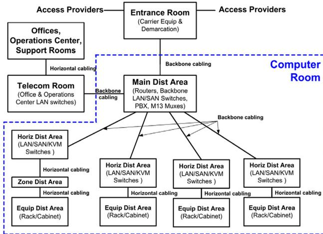
**Fig. 10.** A typical DCN including cabling system.
