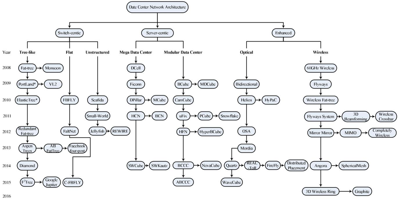
**Fig. 12.** A chronological tree of data center network architectures. Note: Portland\* and ElasticTree\* are not topologies, but are two important improvements to Fat-tree.
