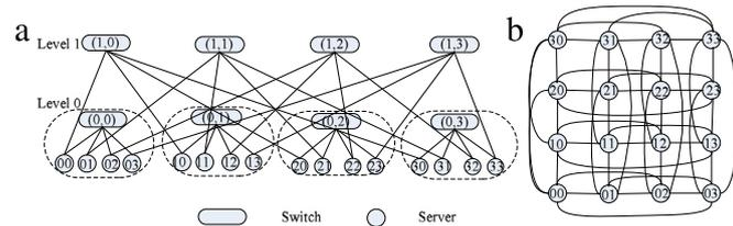
Fig. 30. (a) BCube<sub>1</sub> with  $n = 4$ . (b) A generalized hypercube equivalent to BCube<sub>1</sub> with  $n = 4$ .
