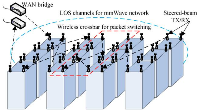
Fig. 43. The wireless crossbar packet switches is configured via LOS channels on top of the server racks.
