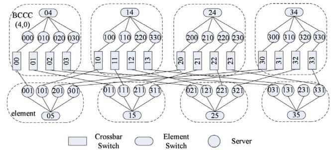
Fig. 34.  $BCCC(4, 1)$  is composed of 4  $BCCC(4, 0)$ s along with 4 elements  $BCube(4, 0)$ .
