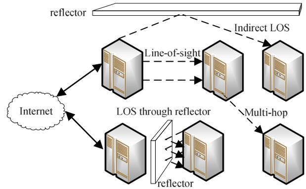
Fig. 40. A wireless data center with 60 GHz links.
