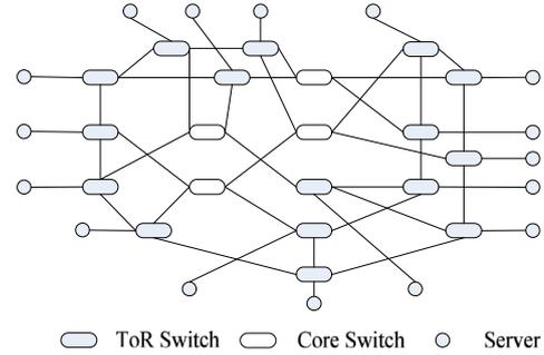
**Fig. 22.** A Jellyfish with 16 servers and 20 4-port switches.
