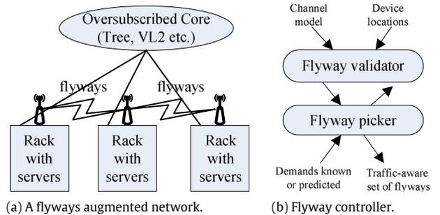
Fig. 41. A flyways augmented network and its controller.
