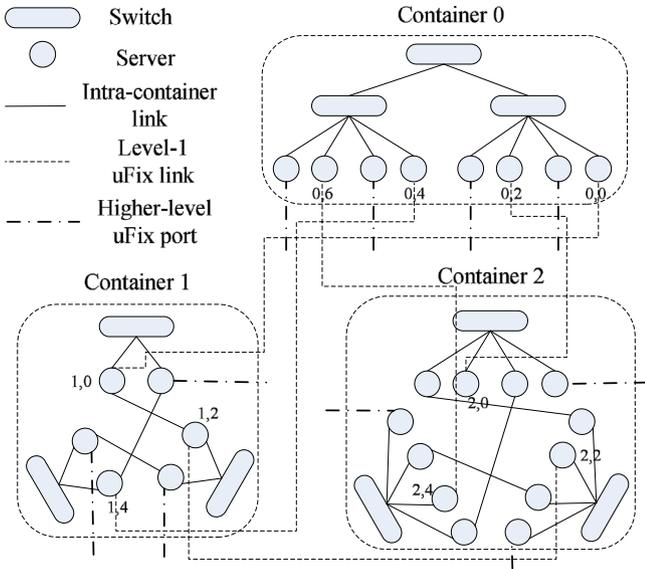
Fig. 32. A 1-level uFix network architecture.
