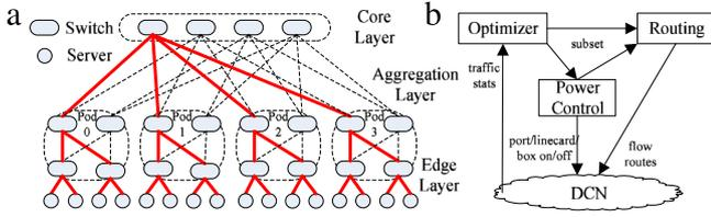
Fig. 14. (a) An example ElasticTree topology. (b) ElasticTree system diagram.
