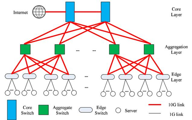
**Fig. 11.** Traditional data center network architecture.
