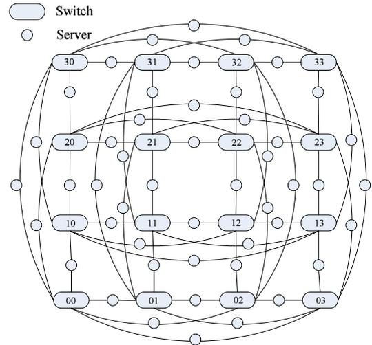
Fig. 28. A 2D SWCube with 4 switches in each dimension.
