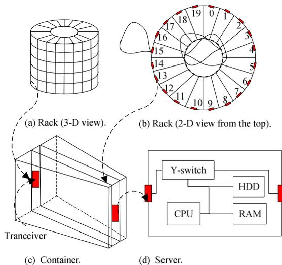
Fig. 44. Rack and server design of Wireless Data Center.
