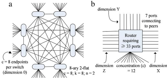
**Fig. 21.** (a) The logical illustration of an 8-ary 2-flat FBFLY. (b) A 33-port router to implement an 8-ary 4-flat with a concentration of 12 (oversubscription of 3:2).
