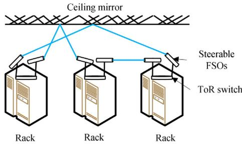
Fig. 39. High-level view of FireFly network.
