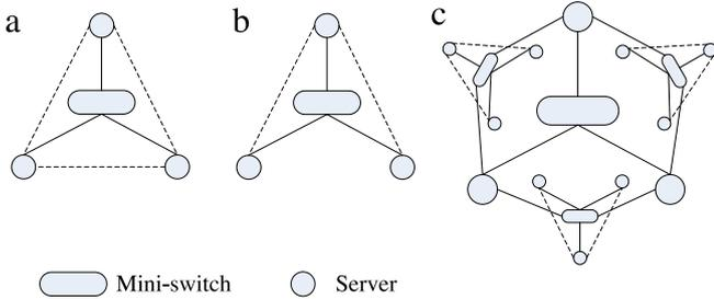
Fig. 33. (a) A Snow<sub>0</sub>. (b) A Cell. (c) A Snow<sub>1</sub>.
