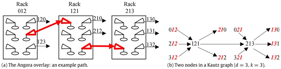
Fig. 46. High-level view of Angora network.
