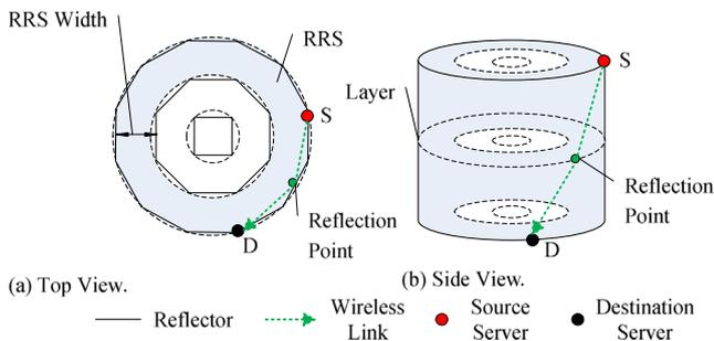
Fig. 48. Top and side views of the 3D wireless ring in Diamond ( $N = 3$  rings and  $H = 3$  layers).
