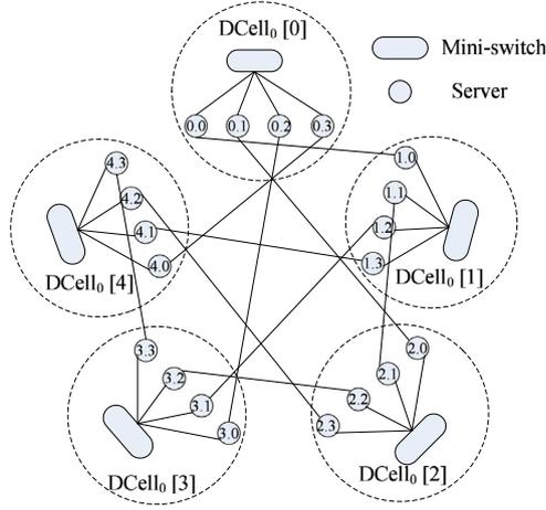
Fig. 23. A DCell<sub>1</sub> network architecture with  $n = 4$ .
