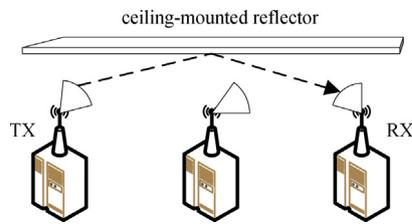
Fig. 42. 3D beamforming.
