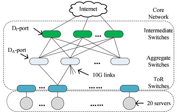
Fig. 16. An example VL2 network architecture.
